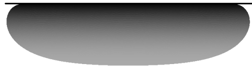
Figure 8: Front view of the actual shape of a large bubble pressed up against a flat plate.
