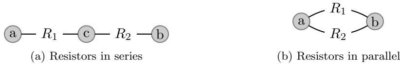
Figure 2: Configurations for resistors in series and in parallel. R_1 and R_2 denote the resistances of the labelled edges.
