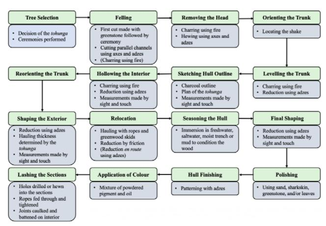
Figure 1. Chaîne Opératoire for the Carving of an Eighteenth-Century Māori Waka Taua Hull, the Human Aspects. (Optional actions are indicated in parentheses).
